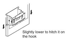
③ Move left the LCD TV to lock it. Make sure that the TV will not fall off.
